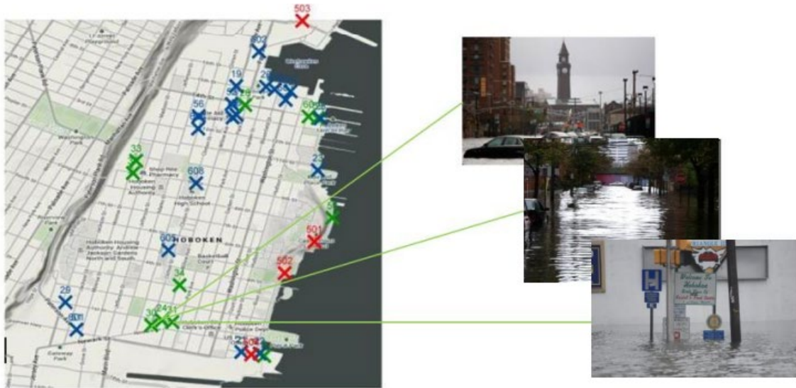
Figure 4-3: Crowdsourcing to Validate Flood Modeling. In partnership with the State, Stevens Institute of Technology is exploring innovative techniques to gather data to inform risk analysis. This photograph is one of many captured both during and following Superstorm Sandy through crowdsourcing. Geo- and time-stamped photos, like this one, allow the State to validate model projections against documented data points, further refining the accuracy of flood modeling to identify areas of increased flood vulnerability.
